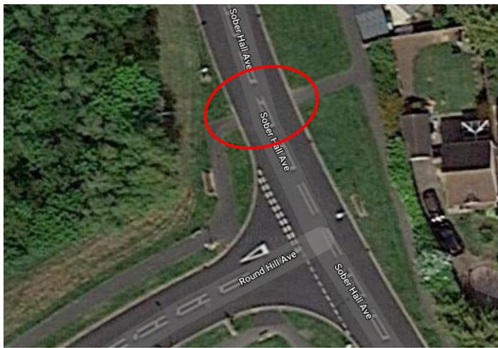
Costs to provide a pedestrian refuge is dependent on the width of the island and the carriageway widening required and is estimated to be in the region of approximately £5,000 - £15,000. Further detailed investigation would be required for a more accurate estimate and to establish its viability should this be a preferred option.
